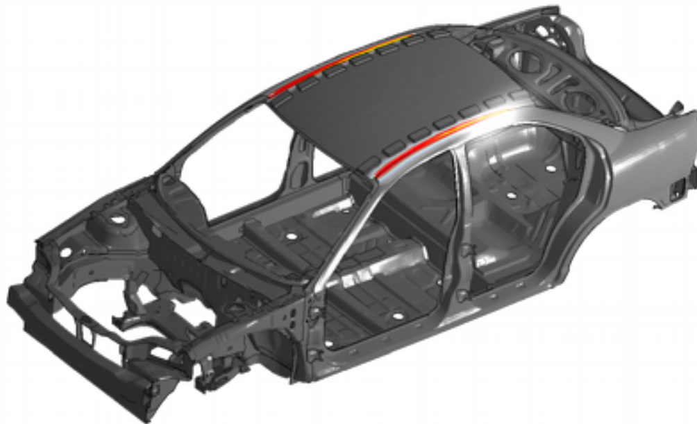
DynaWeld Car: Welding process of the roof
